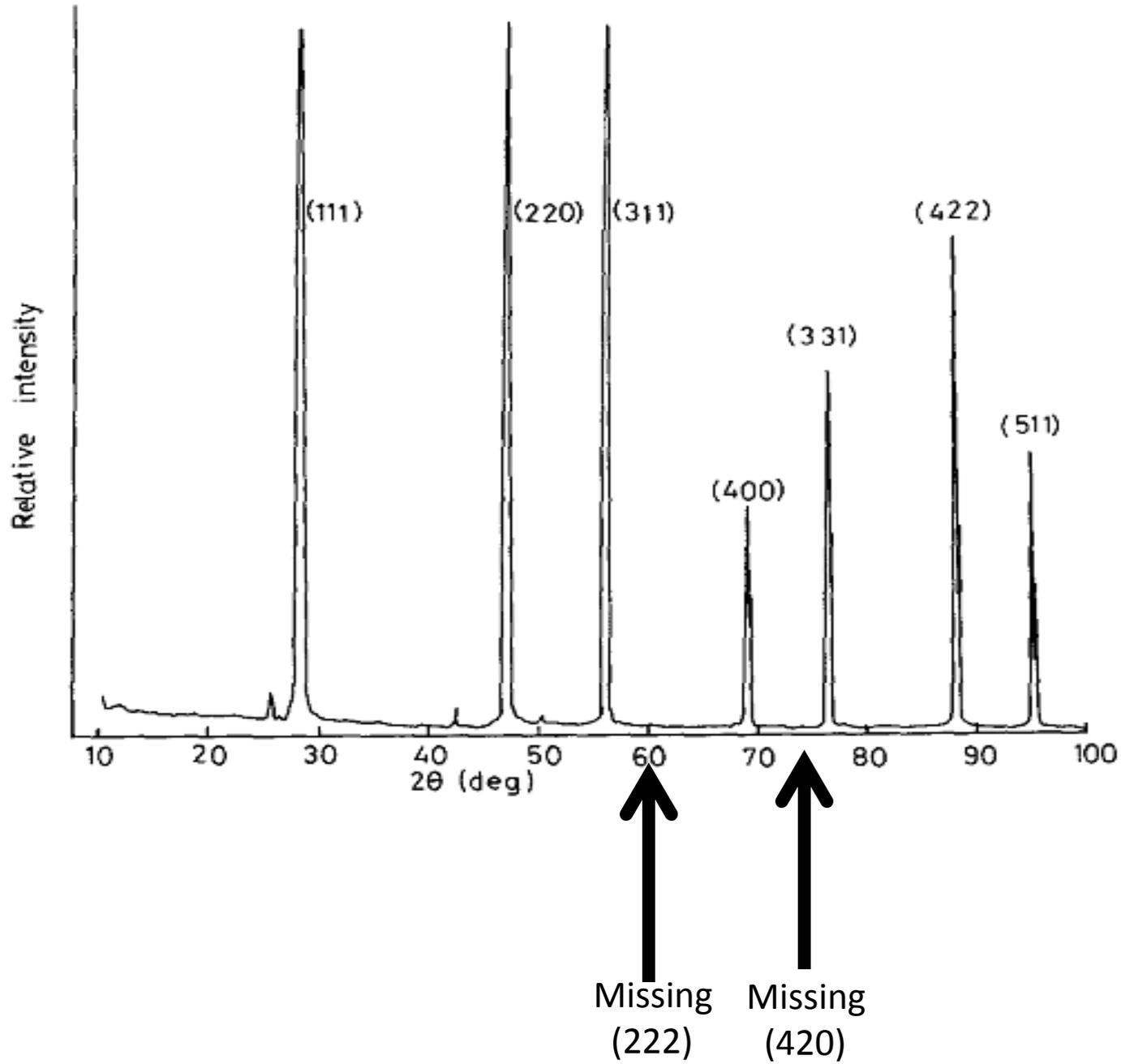
Clean Silicon (Data from Synchrotron)
