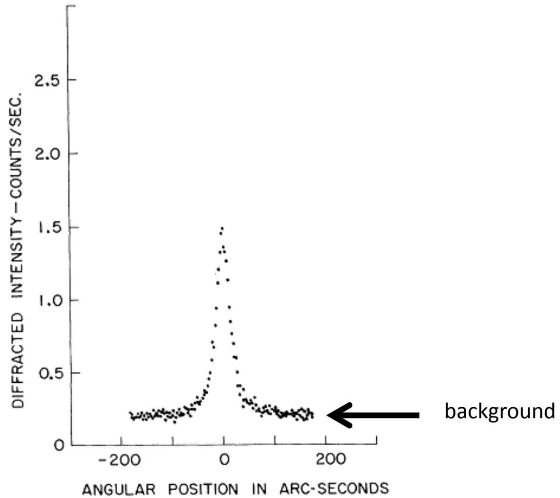
FIG. 1. Typical (222) diffraction profile from a Si crystal
