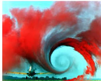
Figure 5: Vortices around an aircraft.
